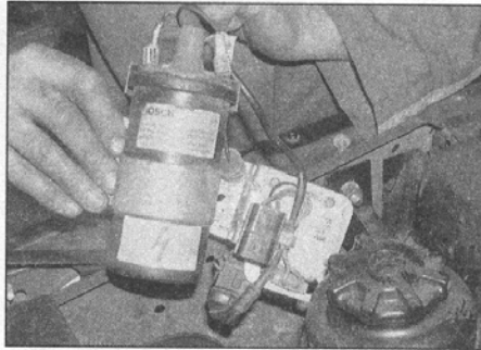
3.4b . . . and remove the coil and amplifier (later model shown)
