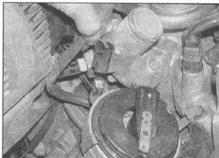
4.4 Disconnect the wiring plug from the distributor body
