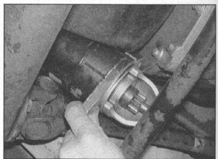
9.9 Removing the starter motor
